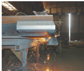
S-100 Torch set with Long slide bar option
