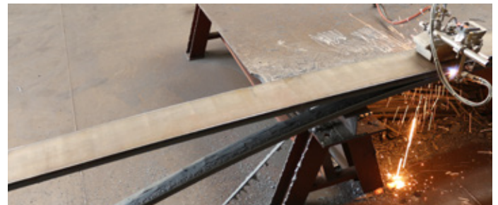
S-100 Torch set with long slide bar and guide roller option
